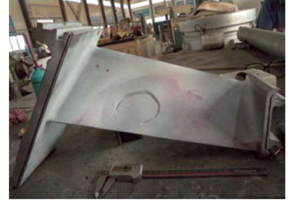
Before Repair – Siemens IN939 Blade
