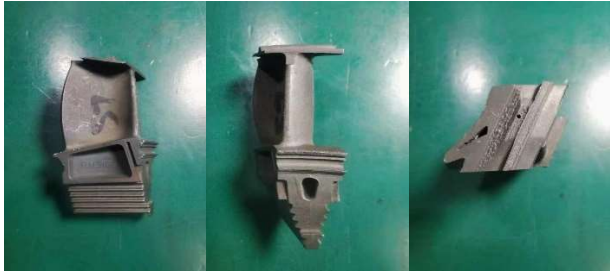
Initial Blade Defect Status
