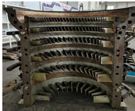
Post-Repair Condition – LP Stator Vane
