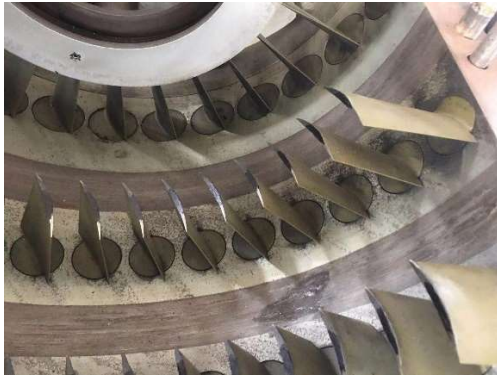
LP Stator Before Repair
