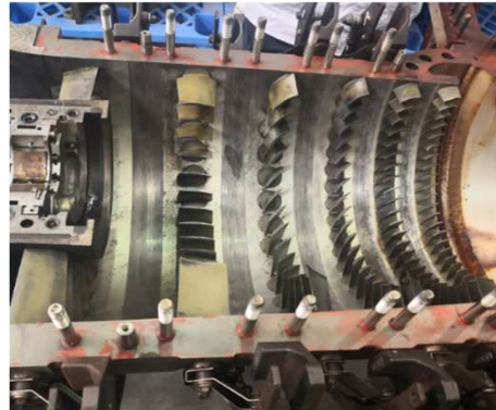
LP Stator Before Repair
