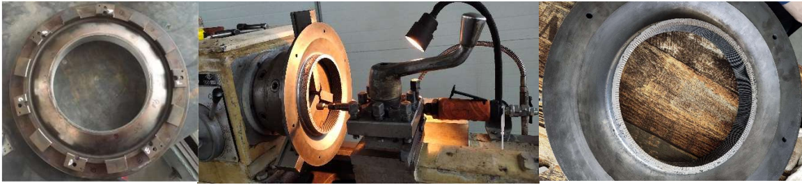
Honeycomb Disk – Before Repair / After Repair
