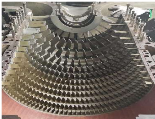
Post-Repair Condition – LP Stator Vane
